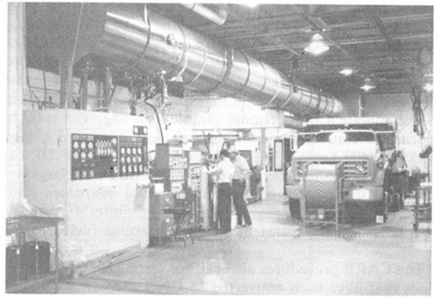
Fig. 3 Heavy-duty chassis dynamometer test setup with GMC 8.2 L truck showing CVS dilution tunnel, analyzers, and control panel
